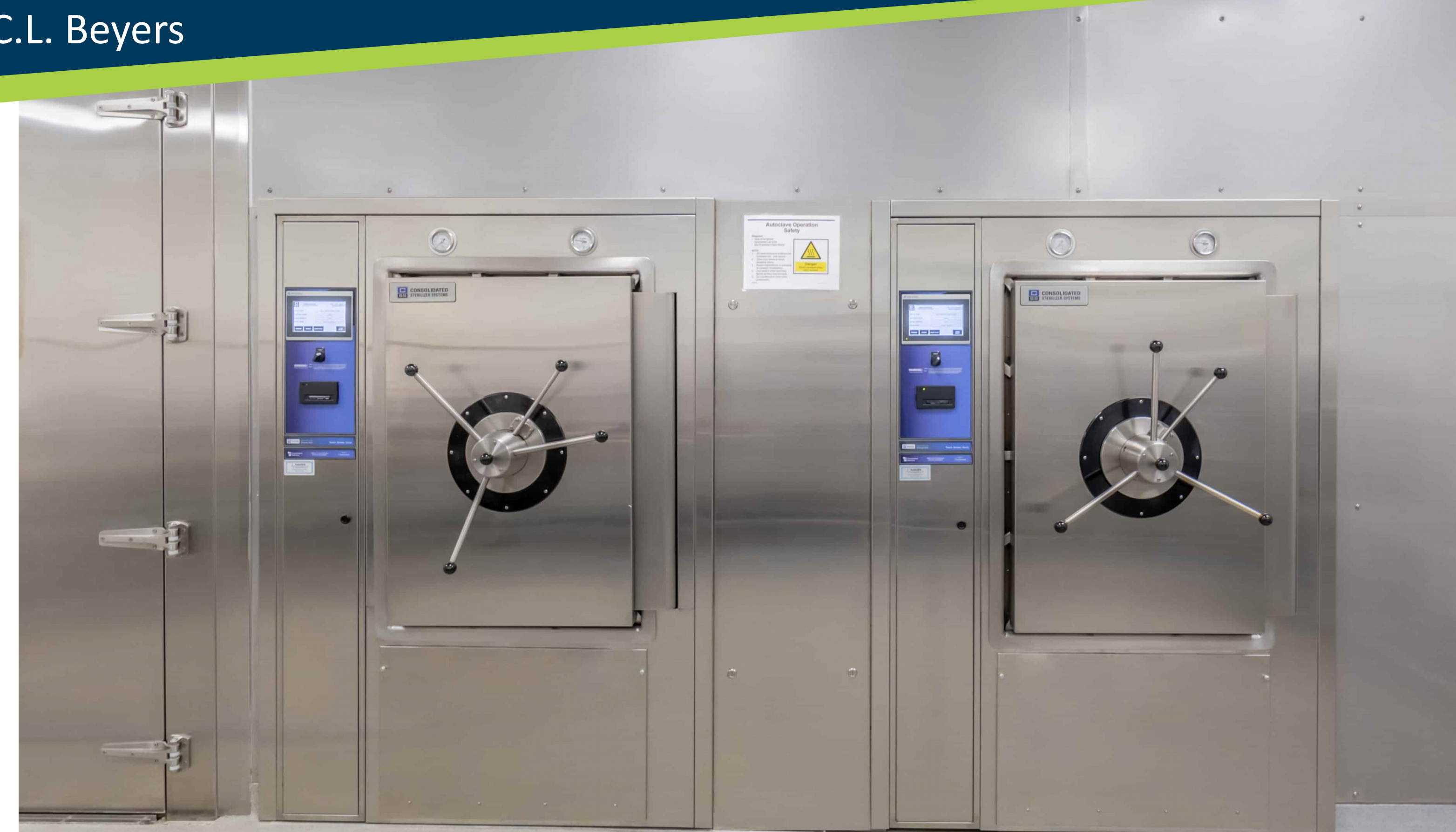
Picture: an autoclave for moist heat sterilization of medical equipment and devices.
